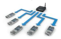
Deploy automatic firmware updates for Philips PocketMemo dictation recorders. The firmware will be updated automatically the next time the recorder is connected to the WLAN adapter.
